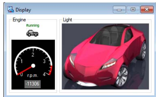
Fig. 8. Inappropriate value on a vehicle simulator display via fuzzing
