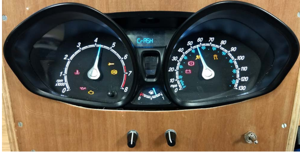
Fig. 9. Crashing a vehicle component as a result of fuzzing
