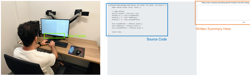
Fig. 2. (Left) The experimental room, with the task displayed on the monitor. The Tobii Pro Fusion Eye-tracker is a thin bar magnetized to a strip at the bottom of the monitor. (Right) A screenshot of one task example, with the Java method displayed on the left of the screen, and the summary writing location in the top right.
